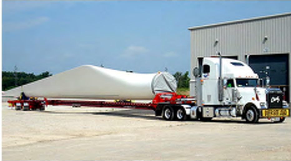
Figure 11 Wind Turbine Blade Delivery Truck
